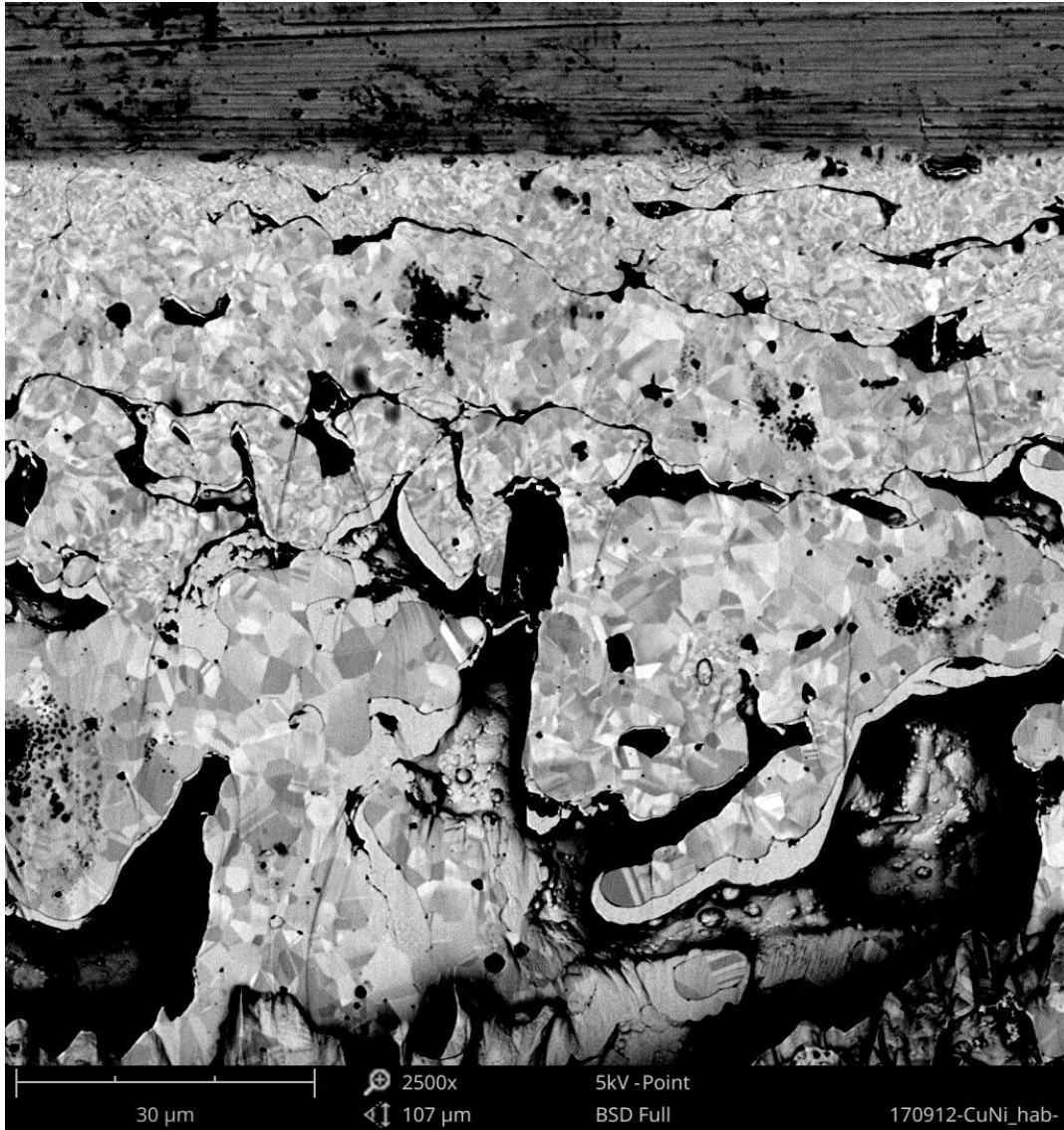
Nickel-copper alloy metal-foam, slope cut @ 30°, 10 kV, 1 hour
