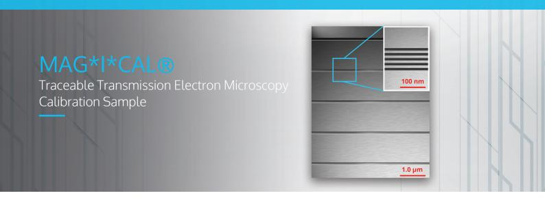
This unique calibration sample is directly traceable to the crystal lattice constant of silicon and can be used to perform the three major instrument calibrations in all Transmission Electron Microscopes (TEMs):
